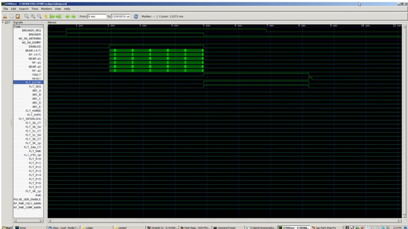
GTKWAVE allows us to arbitrarily shuffle the placement of the signals, so we have done so, putting the bits of interest near the top. Note that we are plotting three separate signals each for the BEAM and RF – we can use these in our custom code to ensure that we haven't lost synch between the data captures on the three boards.
