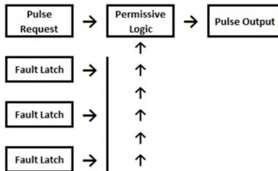
Figure 2. Block Diagram of fault logic permitting pulse pass-thru.
