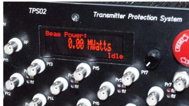
Figure 6. Top level display shows one of several parameters, and the system status in the lower right corner.
